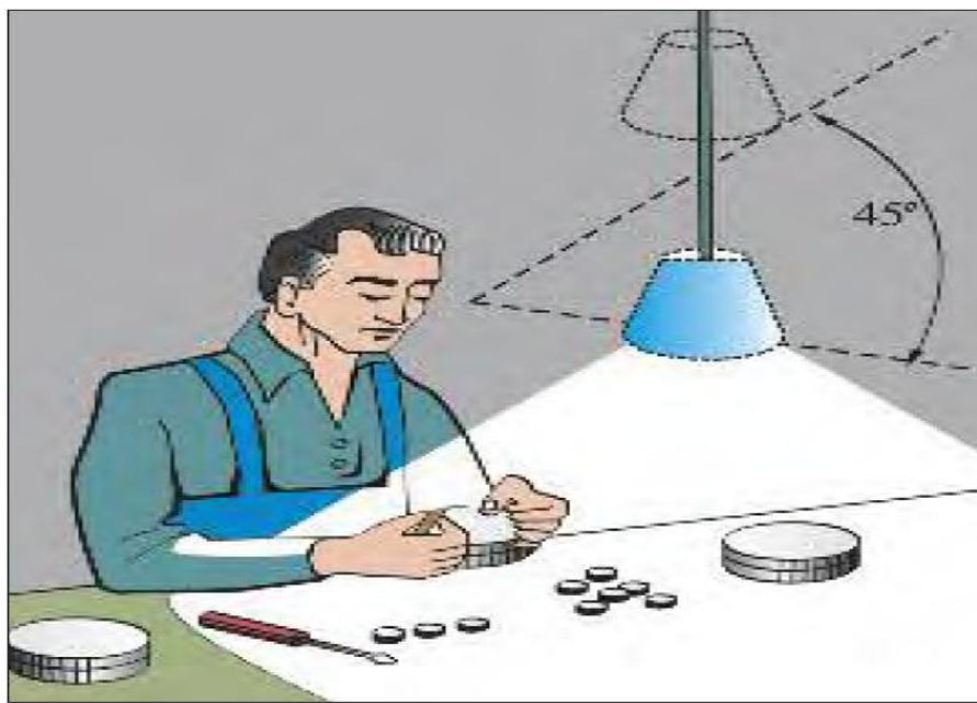
Figure 70a. A shaded lamp should be placed at the appropriate height.
