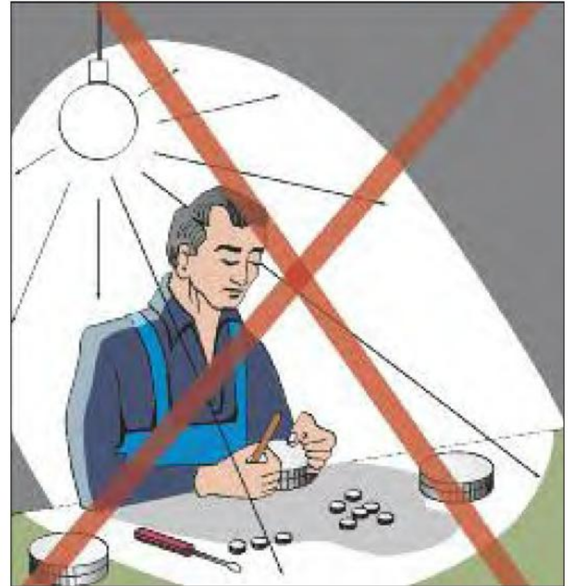
Figure 66c. Sharp shadows make it difficult to work.
