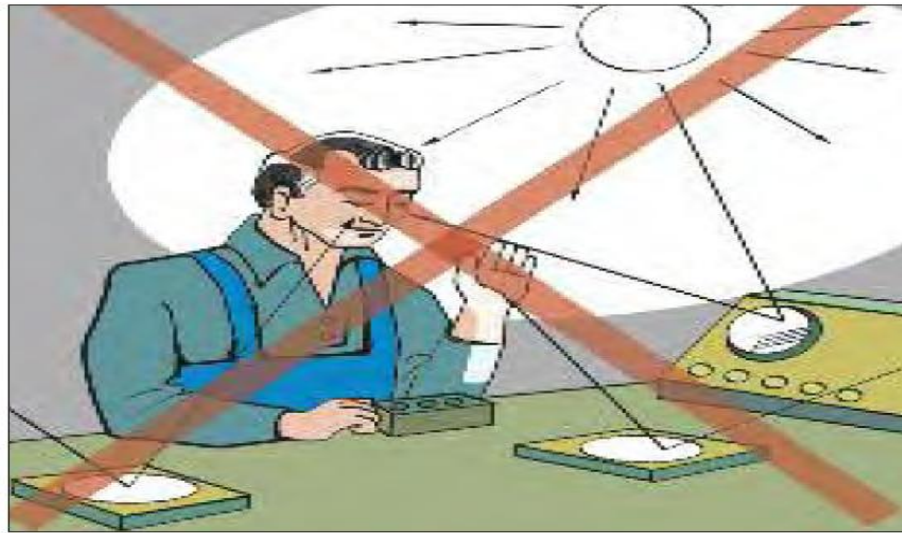
Figure 70c. Reflected (indirect) glare reduces visibility.
